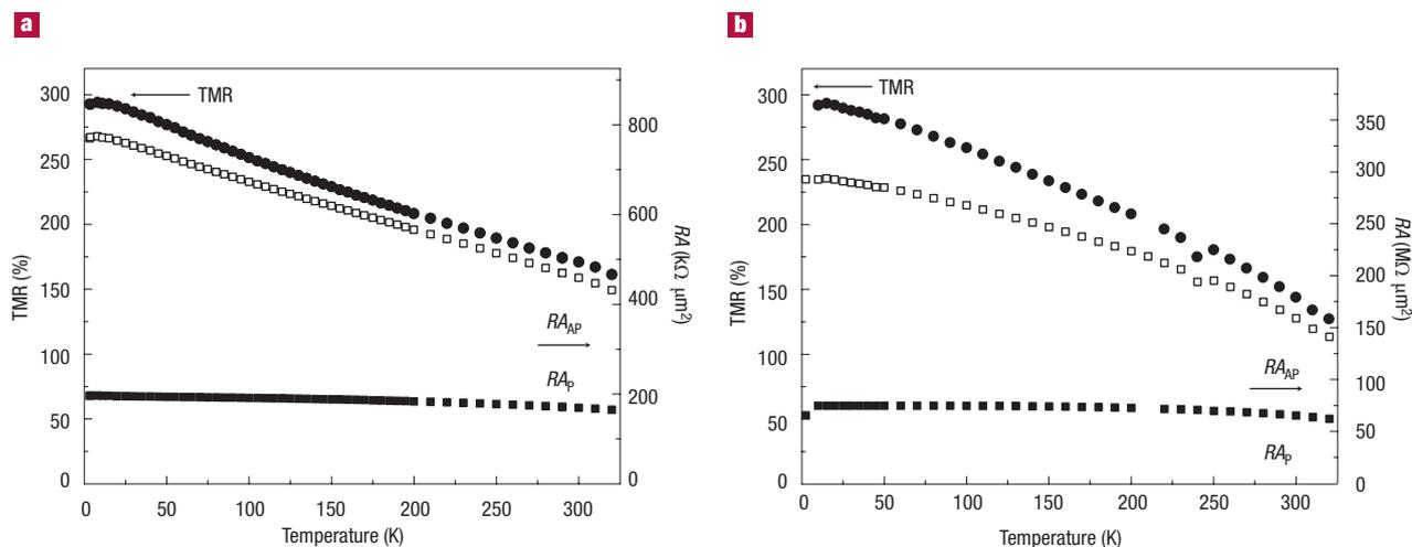
**Figure 4** Temperature dependence of TMR (filled circles) and RA (squares) for the same magnetic tunnel junctions shown in Fig. 1. **a**, Sample from Fig. 1c and d (annealed at 380 °C). **b**, Sample from Fig. 1e and f (annealed at 360 °C) in magnetic fields of  $-100$  and  $+1,000$  Oe to set the state of the junction in the anti-parallel (AP) and parallel (P) states, respectively. The TMR values are extracted from measuring the resistance versus field loop at each temperature.
